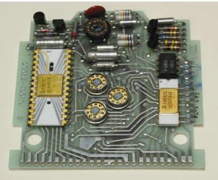
Photo 2: HP-35 Circuit Board With ROM Packages Decapped Photo by Peter Monta
